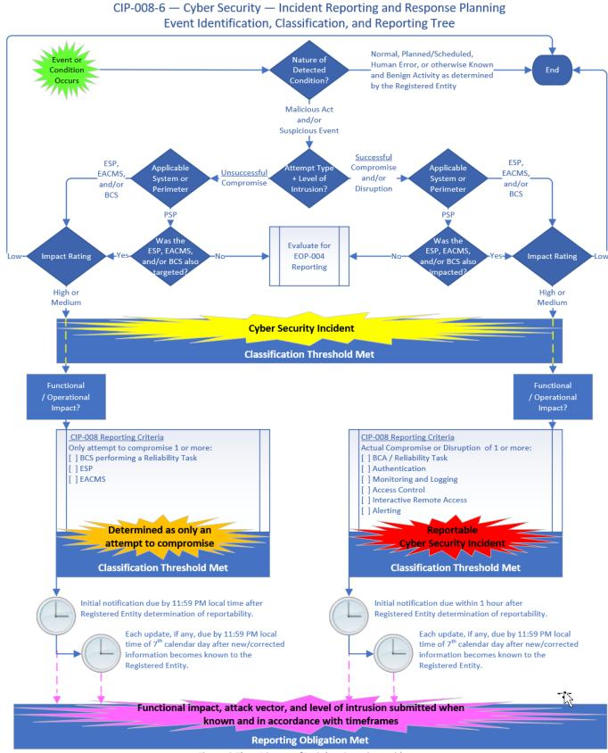
Figure 3 Flow Diagram for Cyber Security Incidents
