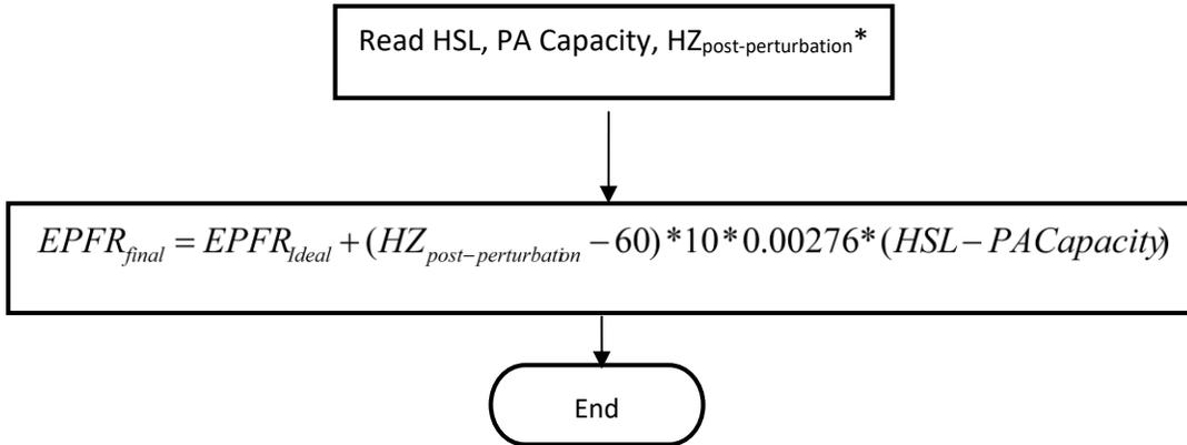
0.00276 is the MW/0.1 Hz change per MW of Capacity and represents the MW change in generator output due to the change in mass flow through the combustion turbine due to the speed change of the turbine during the post-perturbation measurement period. (This factor is based on empirical data from a major 2003 event as measured on multiple combustion turbines in ERCOT.)
