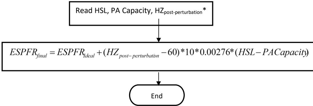
0.00276 is the MW/0.1 Hz change per MW of Capacity and represents the MW change in generator output due to the change in mass flow through the combustion turbine due to the speed change of the turbine during the post-perturbation measurement period. (This factor is based on empirical data from a major 2003 event as measured on multiple combustion turbines in ERCOT.)
