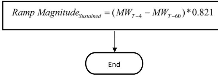
$(MW_{T-4} - MW_{T-60})$  represents the MW ramp of the generator resource/generator facility for a full minute prior to the event. The factor 0.821 adjusts this full minute ramp to represent the ramp the generator would have changed the system had it been allowed to continue on its ramp to T+46 unencumbered.
