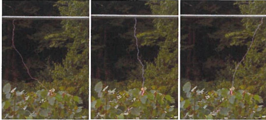
Figure 1-1 Flashovers to Vase, 230 kV, Vertical, Natural Vegetation
