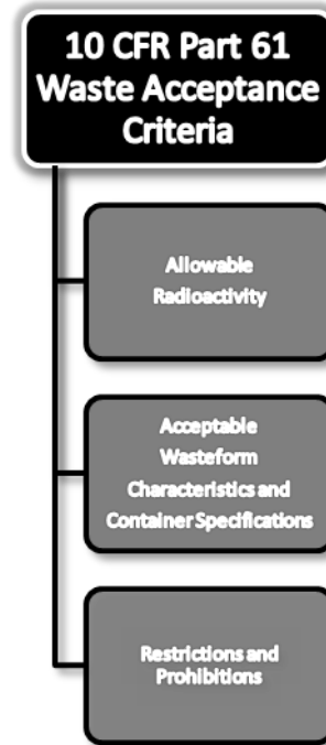
Figure 9-2 Components of 10 CFR Part 61 Waste Acceptance Criteria
