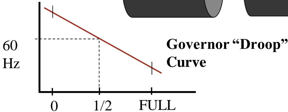
$$\text{Slope} = \frac{\Delta \text{ Freq}}{\Delta \text{ Load}}$$
