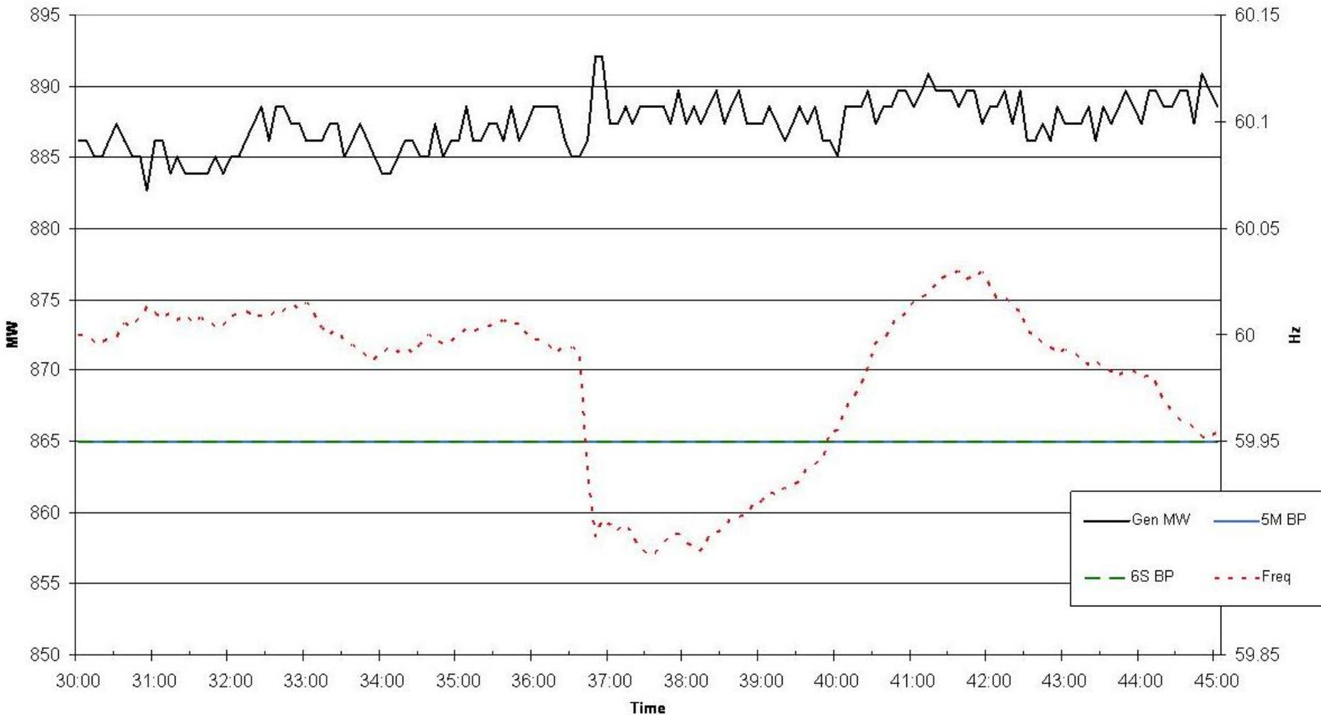
**~900 MW Unit      5% Droop      35 MW Expected      7 MW Actual**
