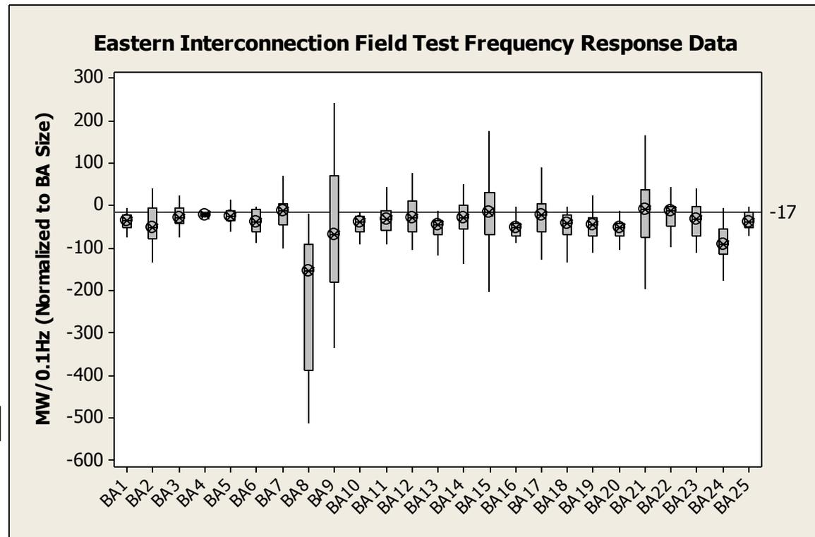
Measurement quality increases when performance is aggregated to the Interconnection level
