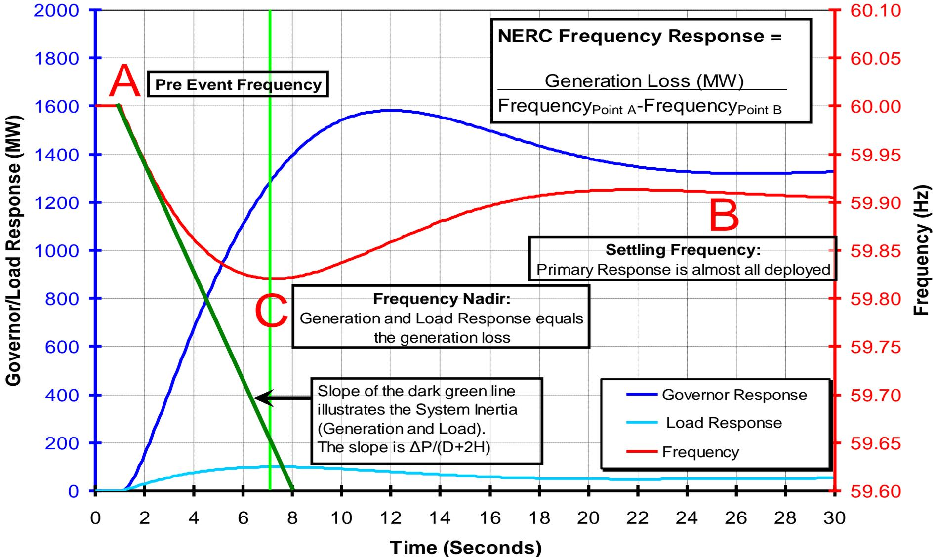
Slope of frequency excursion – determined by the inertia of the system
