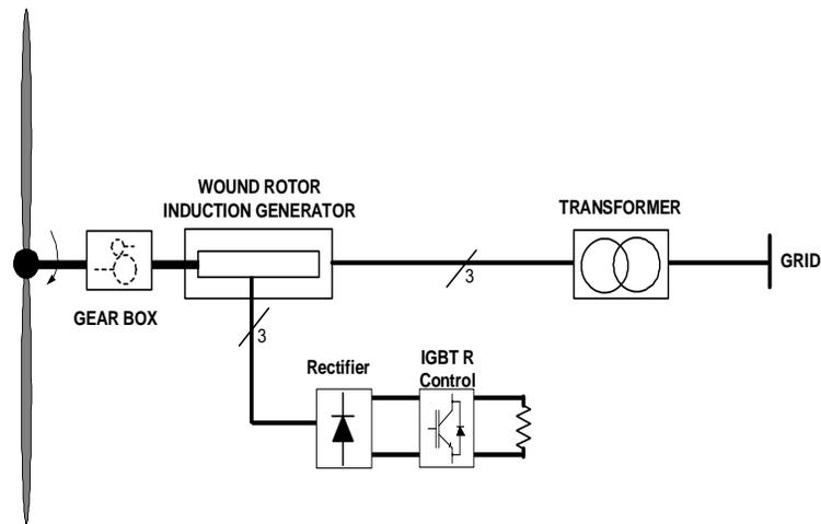
(b) Type 2 Wind Turbine-Generator: Variable Slip Induction Generator<sup>99</sup>
