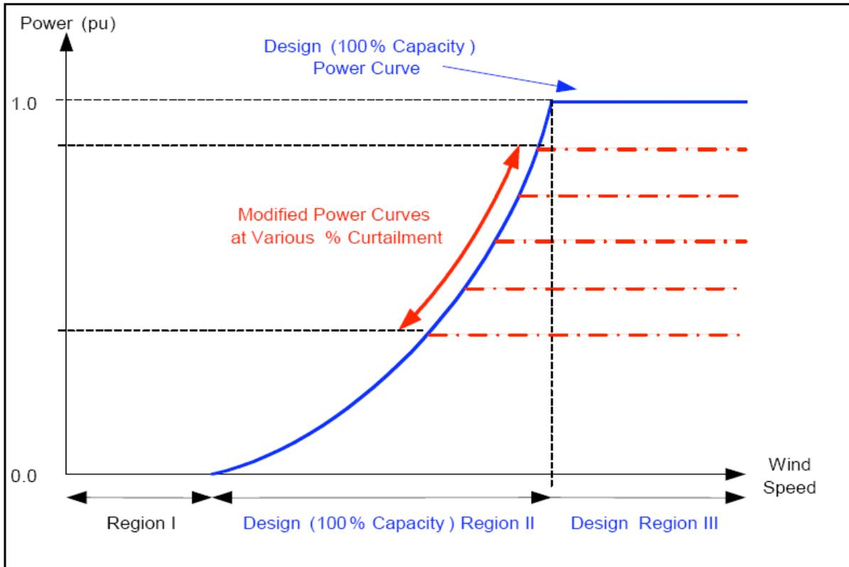
**Figure 2.5: Regulation of Wind Turbine-Generator output using blade pitch control**
